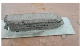
Extruded layered specimen
