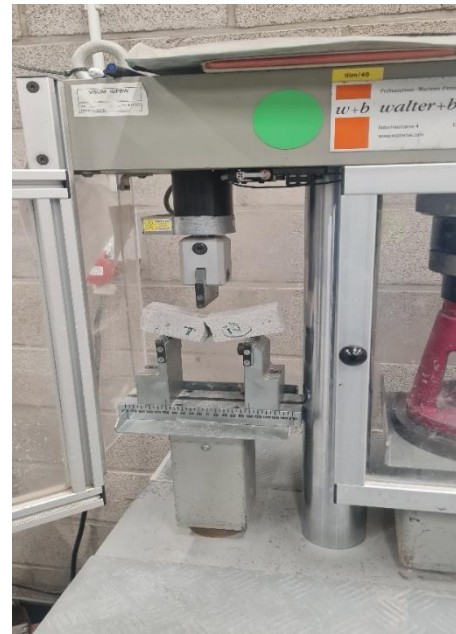
Flexural test (3-point bending) EN 12390-5
