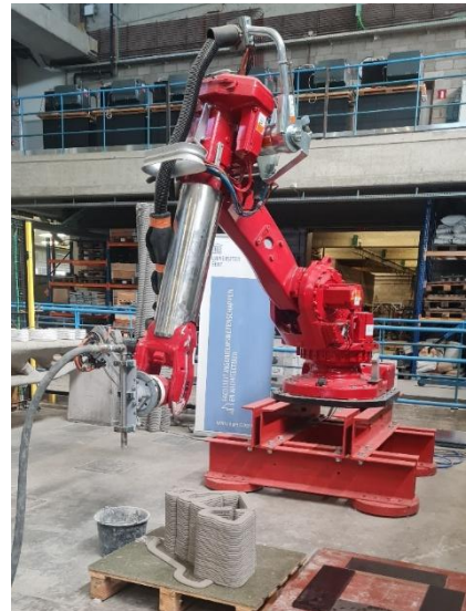
3D-printing with 6-axis Robotic arm at UGent
